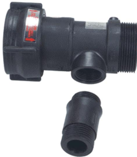
To adjust the amount of foam solution to be educted, the 4060 can also be fitted with a [4064](#) or [4065](#) Variable Percentage Check valve with settings of: OFF, .5%, 1% and 3%. These units must be matched to the flow rate of the eductor.
