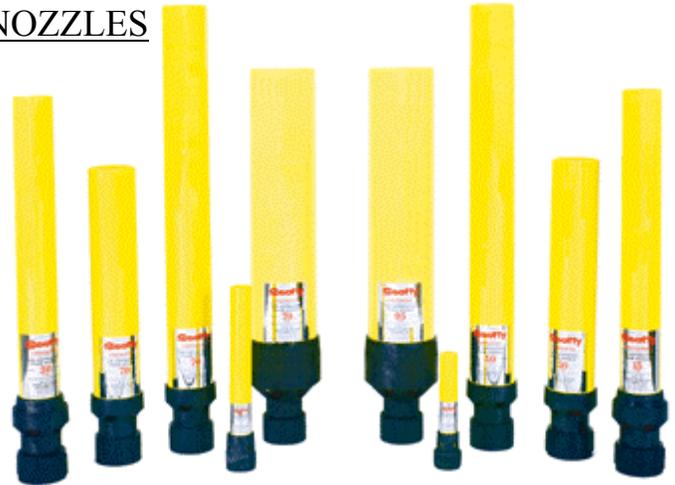
Designed with standard 1.5” NPSH male fire hose threads (3/4” Garden Hose Thread for 4003 and 4005). They can be adapted to a 1.5” coupling on a fire hose by either a Forestry “Quick-Connect” female adapter, a threaded “Stortz” adapter or by a Scotty Double female adapter/connector, 4085 (NPSH) or 4086 (NHT).
