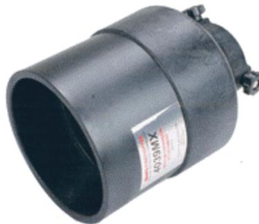
The #4039MX medium expansion foam attachment is designed to fit the Scotty #4037 and #4038 Fog Nozzles. The unit also fits the UFS #1575 Fog Nozzle. Generating a 5” (120mm) thick stream of medium expanded foam it will quickly lay down a foam firebreak for forest and grassland fires. For use against car fires, tire fires, haz-mat or any situation where a thick smothering foam blanket is required.
